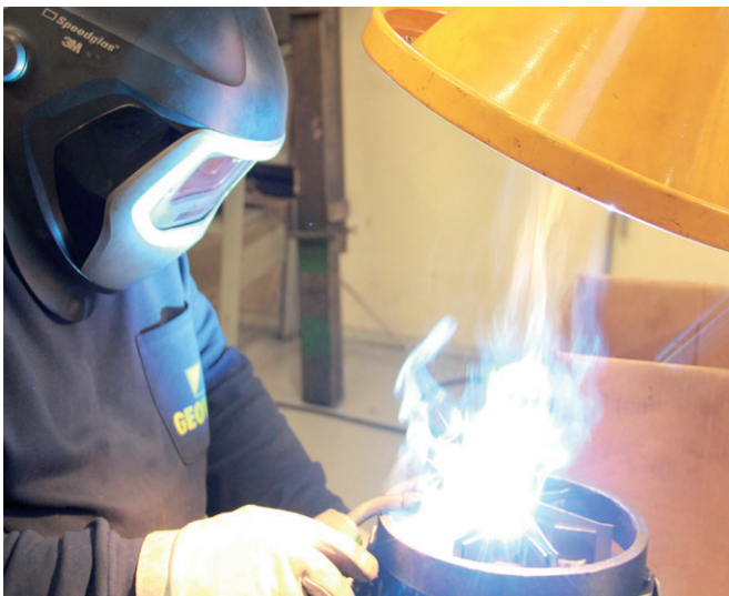
COMPACT arm 1-2m installed and including automatic control devices for automatic start/stop of the fan and motor damper.
