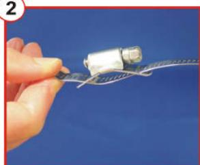
2. Slip the housing over the band with 3cm protruding.
