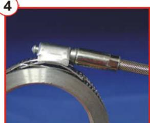
4. Place the Clamp onto the application and tighten the clamp until the required tension is achieved.
