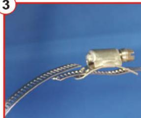
3. Take the other end of the band and position at the rear of the housing, ready to be tightened. Complete the assembly by turning the screw to engage the band.
