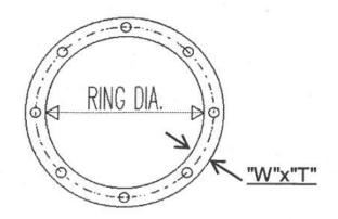
These flanges are compatible with spiral ducting, when used with a top hat spigot (11mm Turn out).
