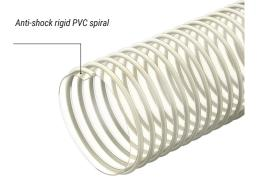
Transparent ether based TPU wall, reinforced with an ivory antishock rigid PVC spiral. Smooth inside, Corrugated outside. Wall thickness from 0.4mm to 0.8mm. Excellent resistance to abrasion and flexion as well as to microbes and Hydrolysis, this hose features high mechanical properties. Light and extremely flexible. Food grade according to FDA REg. Cfr 21- 17.2600 and to EU Reg.
