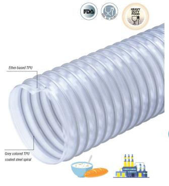
Translucent ether based food grade TPU hose reinforced with a grey coloured TPU coated high adhesion steel spiral. The wall material is permanent antistatic (R<10° Ohm/m).
