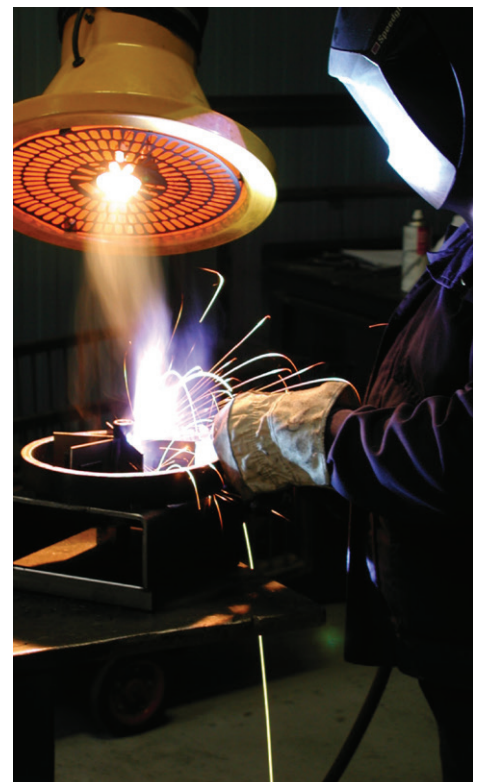
The Wing arm can be offered with built-in light, start/stop switch, manual or motorized damper.
