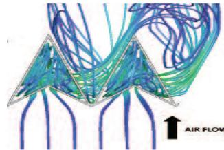
Consequently the static pressure increases only slowly with the accumulation of paint, enabling a uniform airflow around the parts that are being coated, and more importantly clean air
