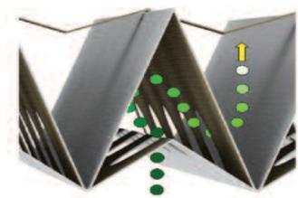
The forward momentum of the rapidly moving droplets separates them from the air stream which makes four quick and violent directional changes and so, deposits the droplets into the deep interior
